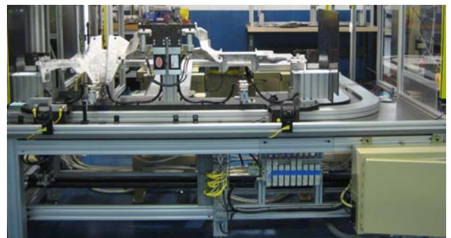
Cam Cover Leak Test
